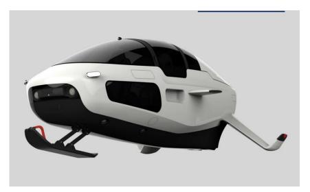
DeepSeaker DS1 is capable of diving to a depth of 50 - 100 meters, depending on the mode. To go underwater, it is necessary to fill the inflatable tank that plays the role of a ballast tank.
